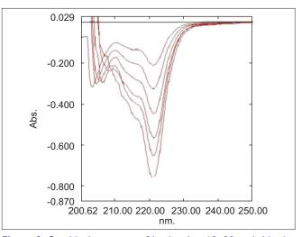
**Figure 2:** Graphical spectrum of Lopinavir at10–30  $\mu$ g/ml in the first-derivative ultraviolet spectrum
