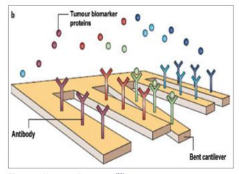
Figure 5: Nanocantilever array<sup>[26]</sup>
