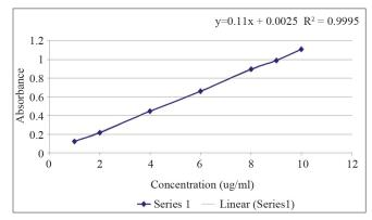
Figure 2: Calibration curve of TCBZ
