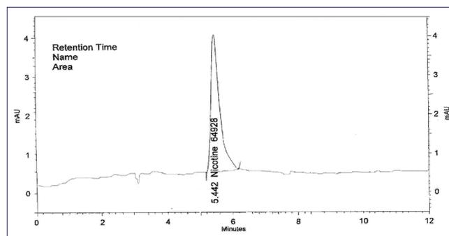
Figure 2: Chromatographic tracing of nicotine extract from untreated root section
