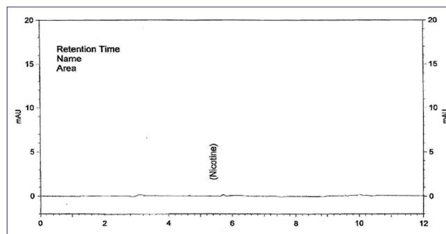
Figure 3: Chromatographic tracing of nicotine extract from treated root section
