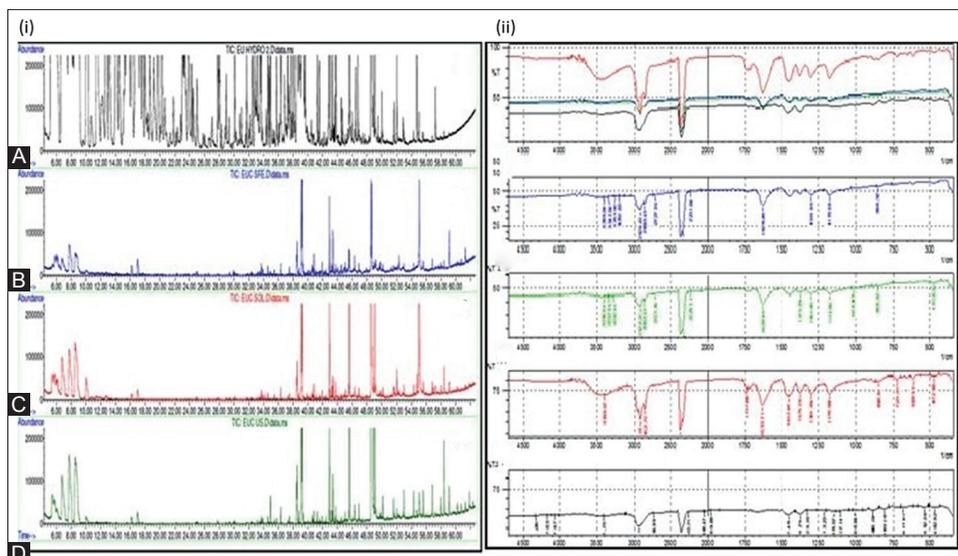
**Figure 4:** (i) GC-MS Comparative chromatograms of different oils of *E. globulus* L. extracted using different extraction techniques (A) SFE oil, (B) Hydrodistilled oil, (C) Solvent extracted oil, (D) Ultra sonication oil. (ii) Comparative spectra of different oils of *E. globulus* Linn. Extracted using different extraction techniques (A) Hydrodistilled oil, (B) Ultra sonication oil, (C) Solvent extracted oil, (D) SFE oil
