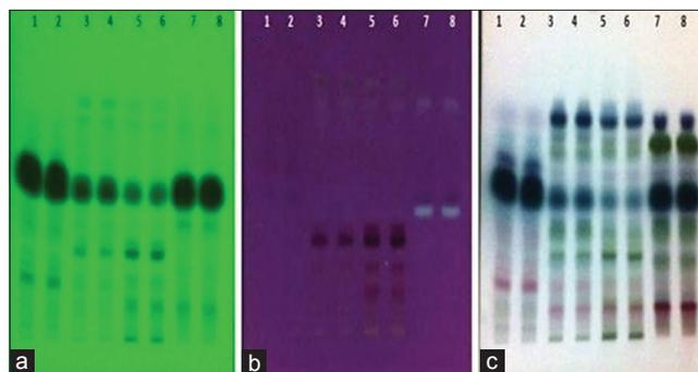
**Figure 1:** HPTLC fingerprint of different oils of *E. globulus* extracted through different techniques [track 1-2: Hydrodistilled oil, 3-4: Solvent extracted oil, 5-6: Ultra sonication oil, 7-8: SFE oil] visualized at (a) 254 nm, (b) 366 nm, (c) Day light after derivatization using anisaldehyde sulphuric acid reagent
