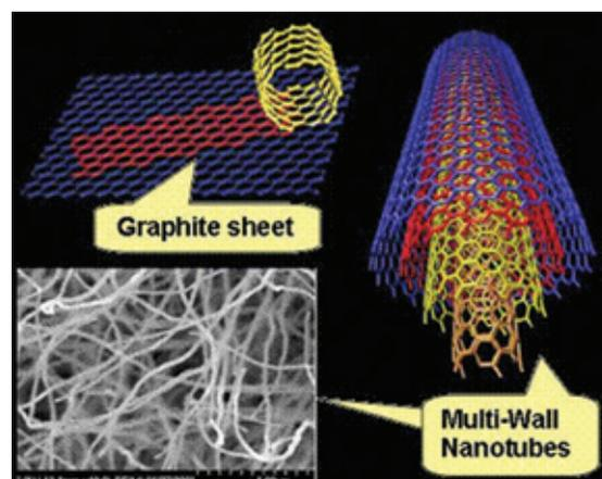
Figure 2: Nanotubes<sup>[38]</sup>
