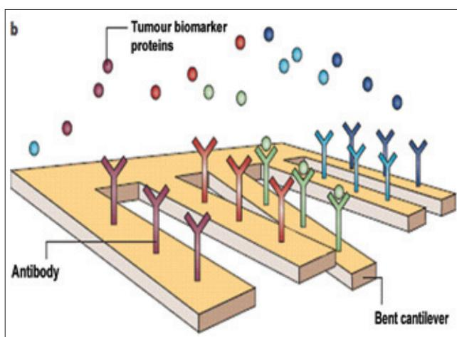
Figure 5: Nanocantilever array<sup>[26]</sup>
