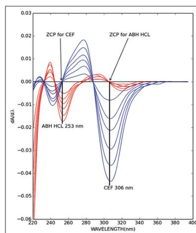
**Figure 2:** First order ultraviolet overlaid spectra in the linearity range of cefixime trihydrate (5–35 µg/ml) and ABH (3–10.5 µg/ml)
