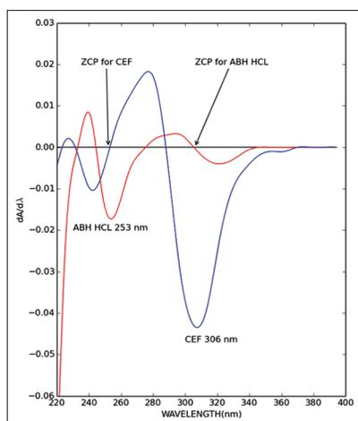
**Figure 1:** First order ultraviolet overlaid spectrum of cefixime trihydrate and ABH showing the zero crossing points of each drug
