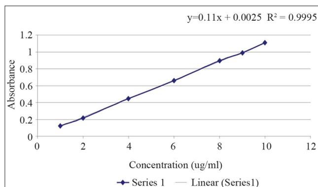
Figure 2: Calibration curve of TCBZ
